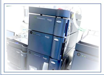
In principle, all classic detectors for LC are available for detection. This includes mass spectrometry as well as UV and fluorescence detectors.
